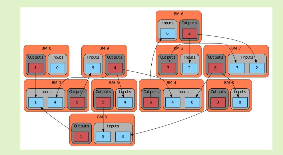
A graphical rappresentation of how to implement a distributed system of BondMachines. The communication among devices follows the very same approch as the communication among cores in a single device.
