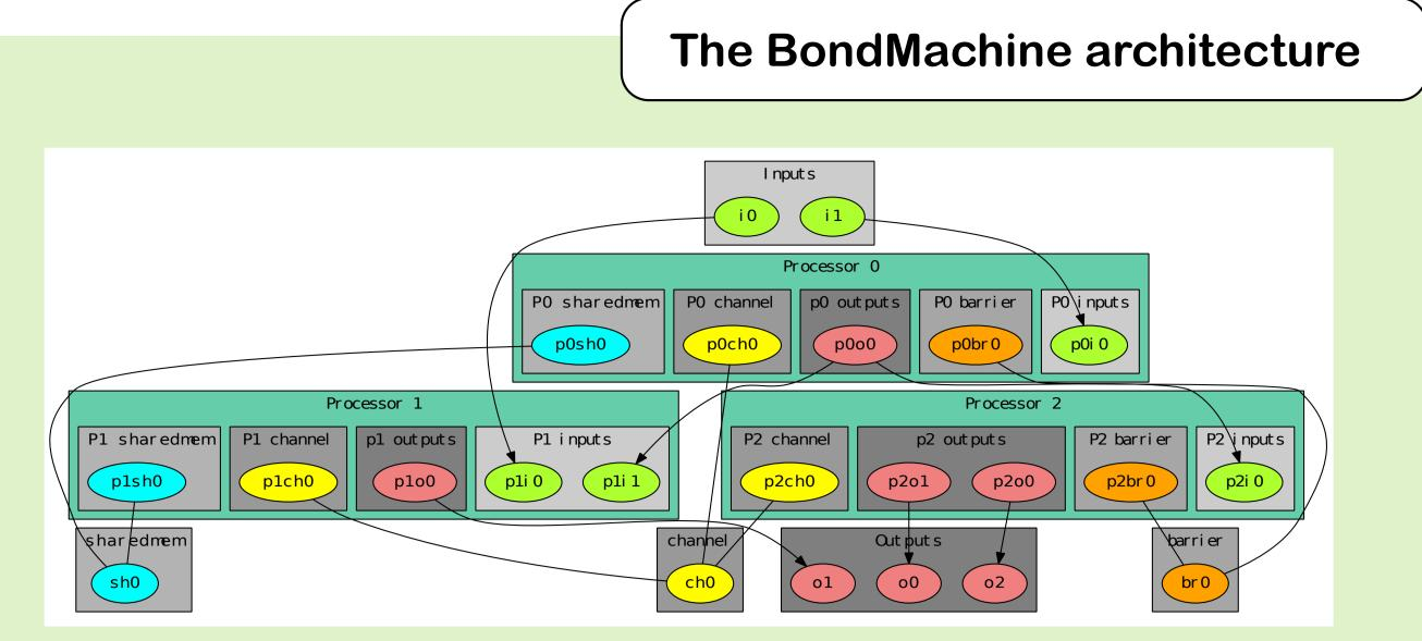
A complete example of the BondMachine architecture. It consists of two inputs and tree outputs interconnected between the input/output registers of the processors. Shared objects, such as memory, Channel and Barrier, are connected among the processors.
