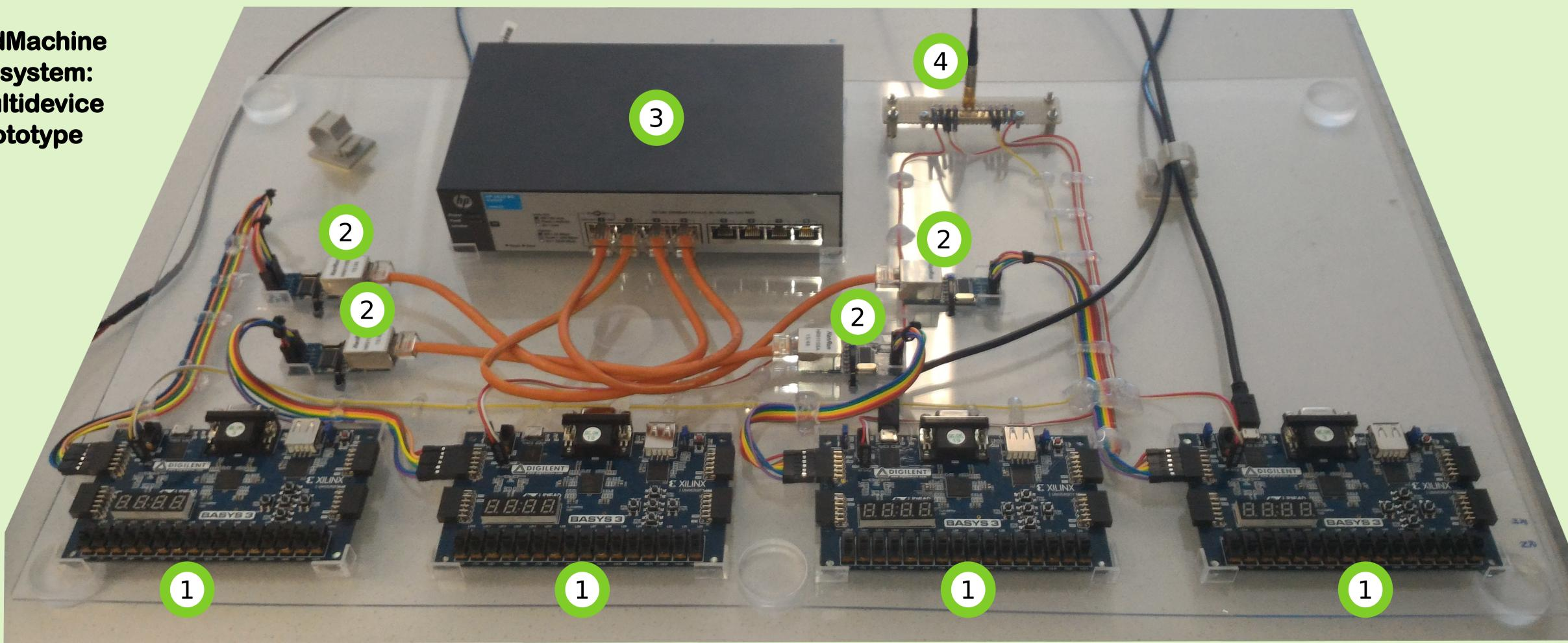
The prototype shown in this picture is composed of 4 FPGA evalution board (1) equiped with SPI ethernet dongles (2) that are connected throught a switch (3). The board are connected to a power supply (4).
